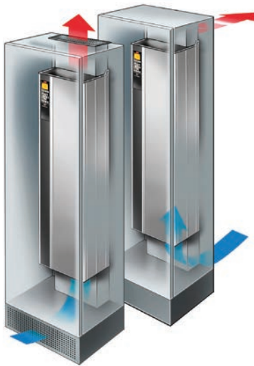
The unique back channel cooling concept transfers up to 90% of heat away from the room. This can result in sizable energy savings by greatly reducing air conditioning requirements.
