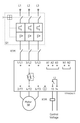
Example 3 - MCD 201 installed with circuit breaker, overload and line contactor.
