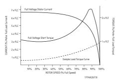
Motors with almost identical full speed characteristics often vary significantly in their starting capabilities. Locked rotor currents range from as low as 500%, to in excess of 900% of motor FLC. Locked rotor torques range from as low as 70%, to highs of around 230% of motor full load torque (FLT).
