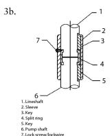
With a keyed coupling insert the key into the pump shaft. Lower the sleeve over the pump shaft, to approximately 1.0 in (25.4 mm) below the top of the shaft. Then lower the lineshaft until it touches the pump shaft. Insert the split ring into the grooves of the pump shaft and lineshaft. Raise the sleeve until it covers the split ring, then insert the key into the lineshaft. Raise the sleeve to
