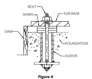
Bolts should be sized and located in accordance with the dimensions given on the Certified Pump Outline Drawing, if provided. The pipe sleeve allows movement for the final positioning of the foundation bolts to conform to the holes in the sub base flange. See Figure 3.
