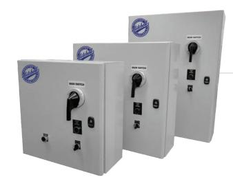
A full voltage starter controls a pump motor with one contactor that closes the power circuit to turn the motor on and opens to turn the motor off. Across-the-Line Starters offer a lower investment cost for applications requiring a disconnecting means, starting circuitry, and motor overload protection.
